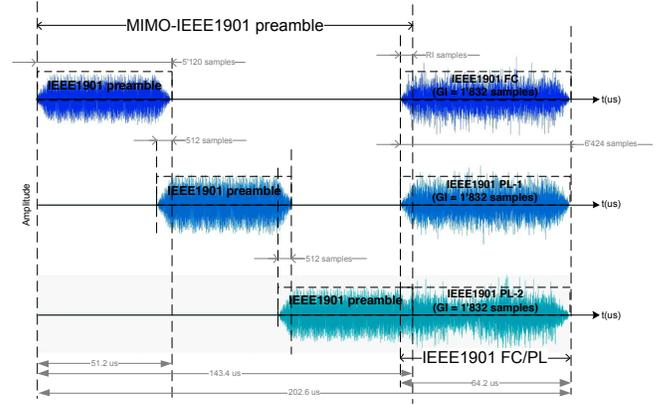
Fig. 2: MIMO PPDU frame format
