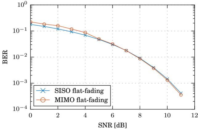
Fig. 4: Bit error rate comparison for flat-fading channels without crosstalk
