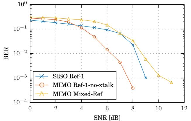
Fig. 5: Bit error rate for fading fading channels: SISO (blue) and MIMO (red) without crosstalk, and MIMO with crosstalk (yellow).
