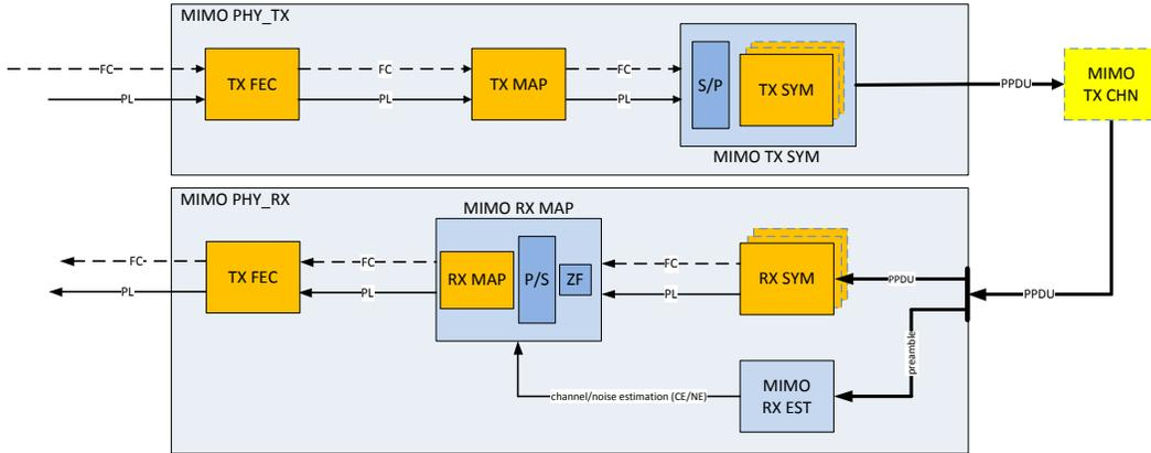
Fig. 1: Architecture of PHY transceiver with MIMO extension
