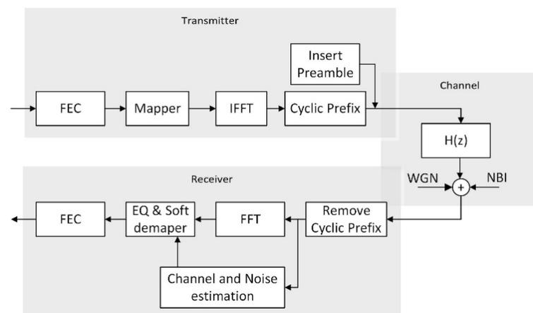
Fig. 1 FFT transceiver
