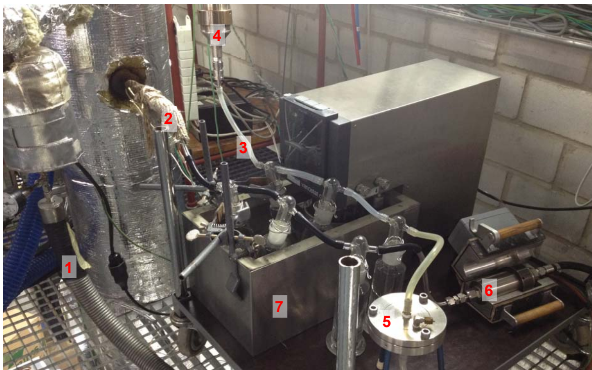
Figure 5.2 Picture of the parallel setup of sampling method 1 and 2. 1) sampling line for gas phase analysis; 2) sampling line method 2; 3) sampling line method 1; 4) heated filter for gravimetric SP determination according to VDI 2066 standard; 5) back up filter to collect COC not trapped in sampling liquid; 6) filter after impingers in sampling method 2 and 7) water bath cooled to 5°C.
