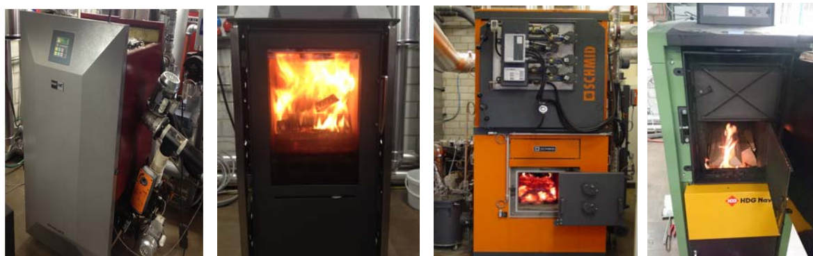
Figure 5.4 Images of combustion devices investigated in this study. From left to right: Pellet boiler, log wood stove, moving grate boiler operated with wood chips, log wood boiler.
